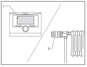
Set the room thermostat or the weather compensator (1) and thermostatic radiator valves (2) as specified in the relevant instructions for these accessories.
